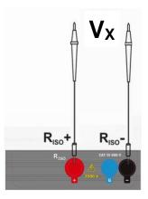
Connect the meter to a voltage source.
