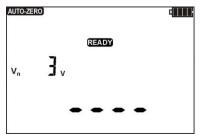
**AUTO-ZERO** message starts to blink, which confirms completion of test leads calibration.
