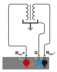
when measuring insulation resistance between one of the cable conductors and the cable jacket, the effect of surface resistances (important in difficult weather conditions) is eliminated by connecting a piece of metal foil insulating the tested conductor with G socket of the meter;
