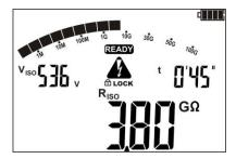
After the measurement is completed or stopped. read the result. The results of all completed measurements will be displayed (even when the measurewas interrupted /stopped e.g. after 60 seconds). When the meter switched into standby mode, the measurement result may be recalled by pressing ENTER.
